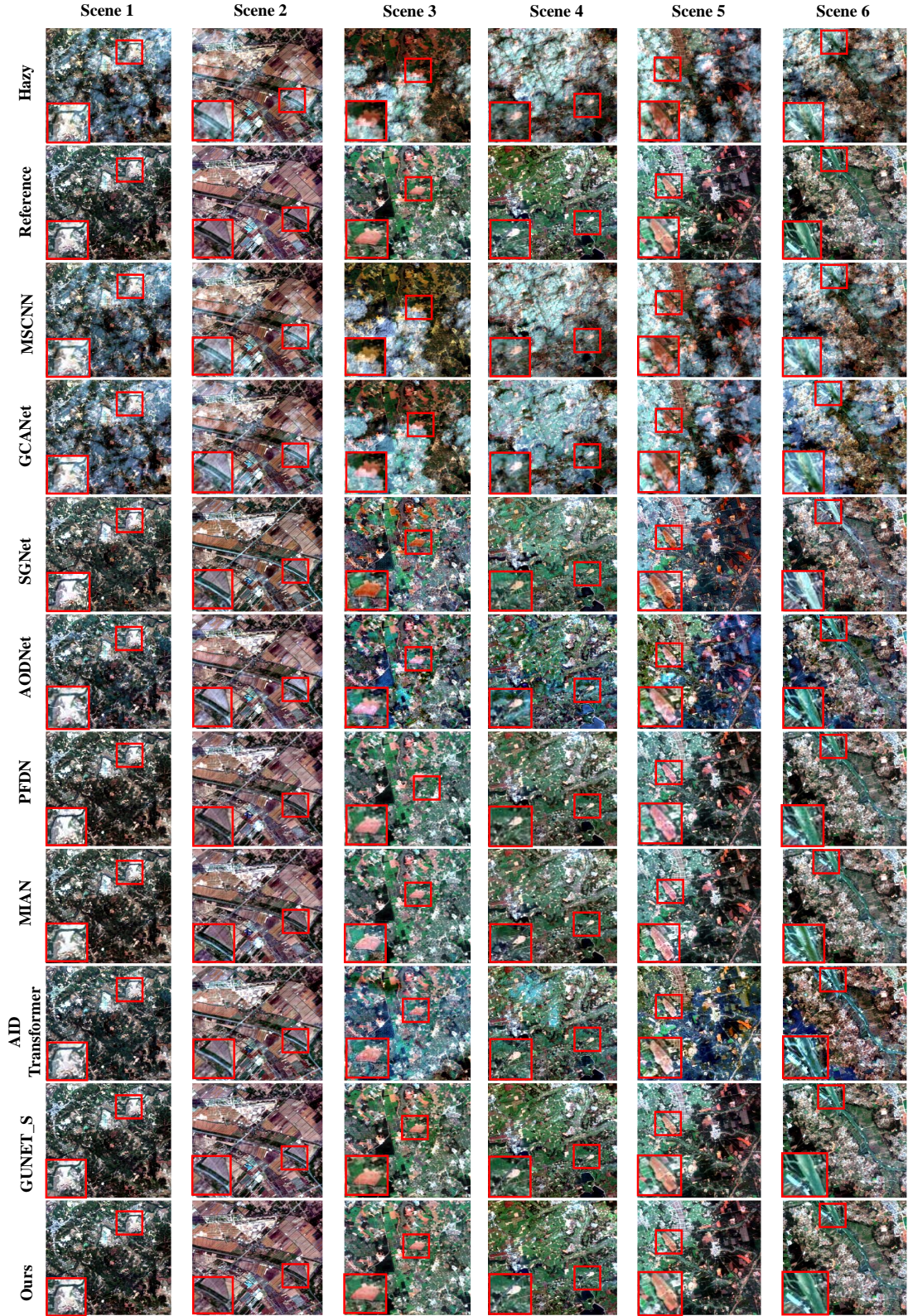
Fig. 4: Haze removal results of six scenes obtained by different methods. The first and second rows are the images contaminated by haze and their corresponding clear images. The third to eleventh rows show true-color composite images of Band 20 (472 nm), Band 35 (536 nm), and Band 65 (664 nm) of the HSI after dehazing.
